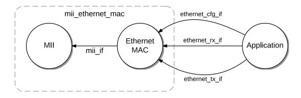
Figure 2: 10/100 Mb/s Ethernet MAC task diagram
