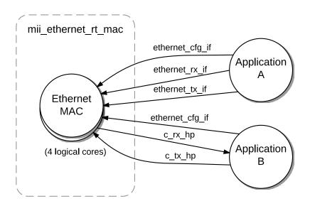
Figure 3: 10/100 Mb/s real-time Ethernet MAC task diagram
