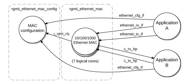
Figure 4: 10/100/1000 Mb/s Ethernet MAC task diagram
